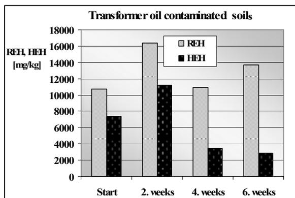
Figure 7. Changes of cyclodextrin extractable hydrocarbons (REH, HEH) in transformer oil contaminated soils
