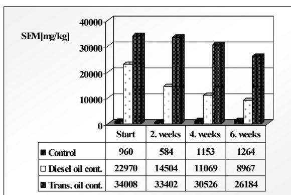
Figure 5. Changes of Solvent Extractable organic Material in static reactors
