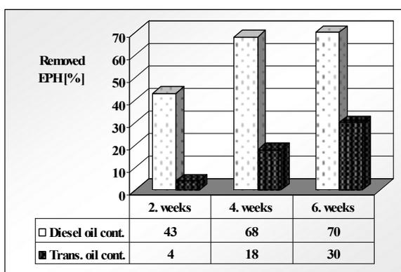
Figure 6. Hydrocarbons-removal in static reactors during the 6-week experiment
