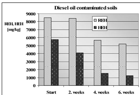
Figure 8. Changes of cyclodextrin extractable hydrocarbons (REH, HEH) in diesel oil contaminated soils
