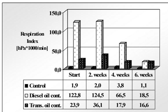
Figure 3. Respiration Index in static reactors measured by "closed bottle" test
