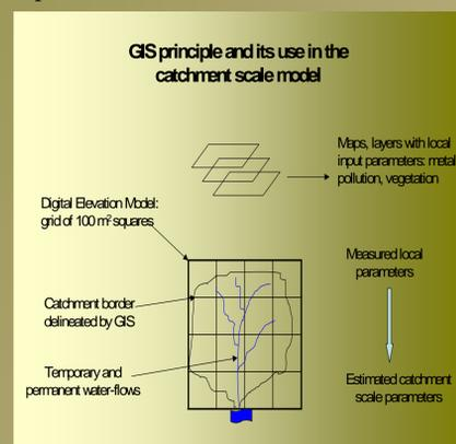
Fig. 3 GIS principle at catchment scale
